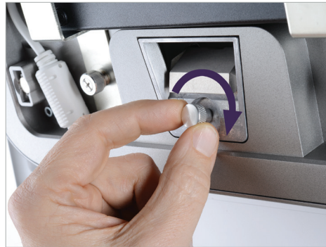
13. Turn the scanner around and tighten the thumb screw to secure the HD screen
